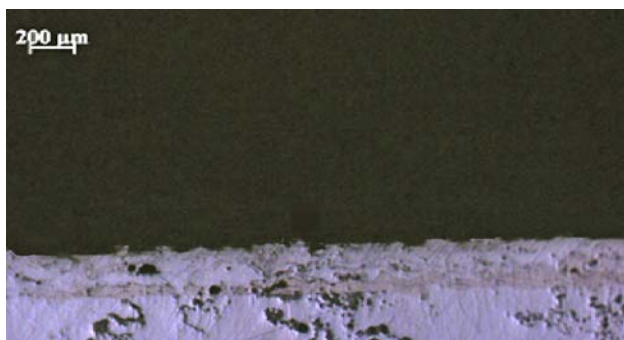
Fig. 14. optical micrograph showing the degradation of coating by corrosion attack in both coating and substrate
