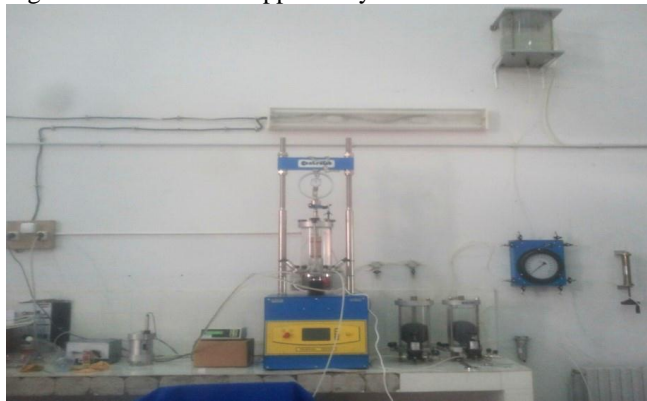
Fig. 15. An overview of triaxial appartus system The various realizable types of test are:
